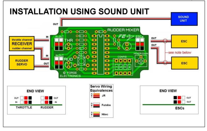
**Note:** if both ESCs have an integral BEC (battery elimination circuit) then one of the BECs should be disabled by removing its red wire from its plug – otherwise the BECs will "fight" each other. If supplying the receiver's 5v supply from a separate battery box and either or both of the ESCs contain integral BECs then the BECs should be disabled. There must be only ONE 5v supply in the installation.
