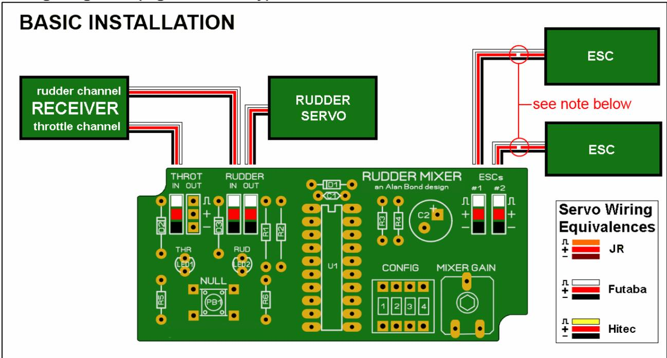
**Note:** if both ESCs have an integral BEC (battery elimination circuit) then one of the BECs should be disabled by removing its red wire from its plug – otherwise the BECs will “fight” each other. If supplying the receiver’s 5v supply from a separate battery box and either or both of the ESCs contain integral BECs then the BECs should be disabled. There must be only ONE 5v supply in the installation.
