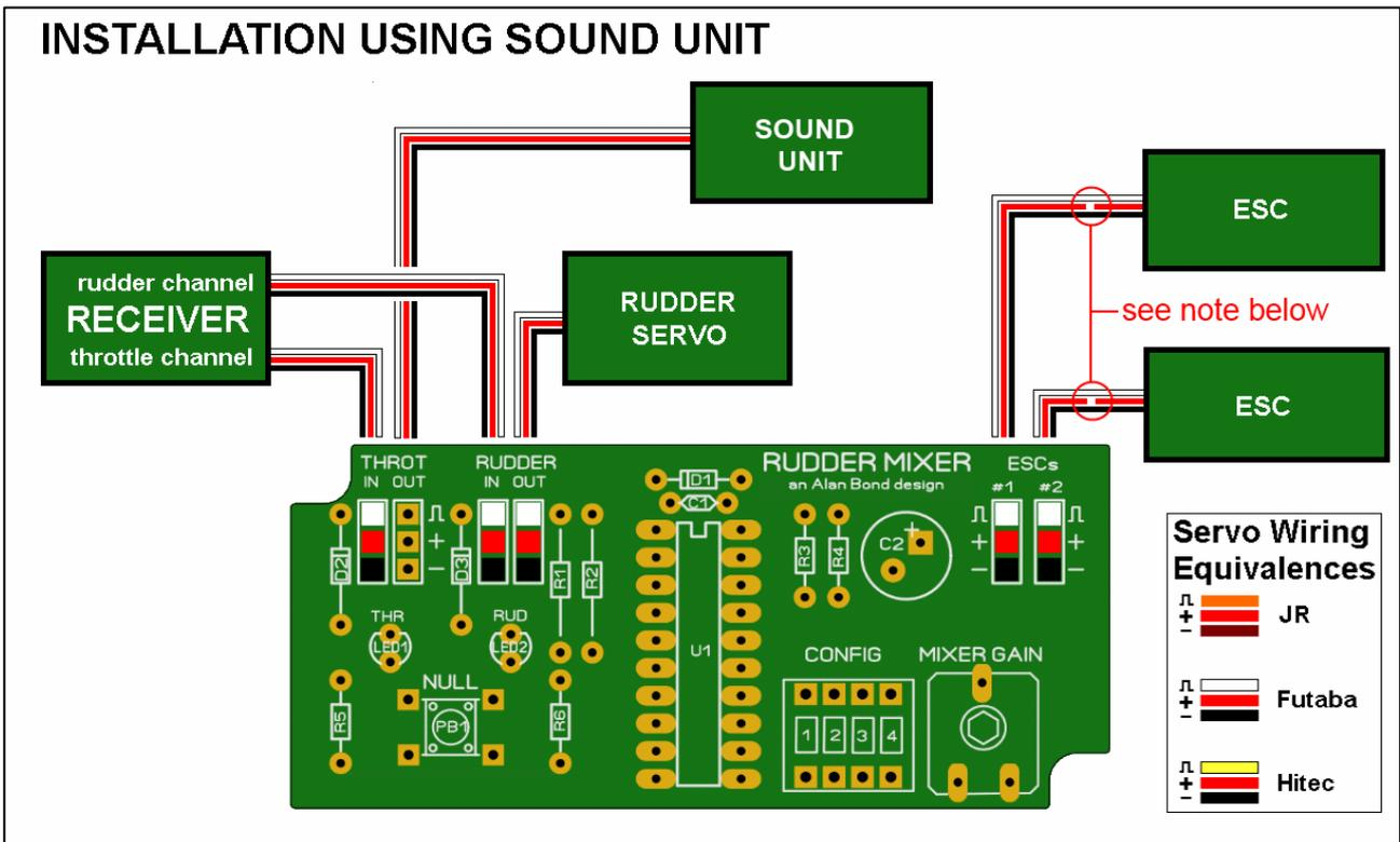
**Note:** if both ESCs have an integral BEC (battery elimination circuit) then one of the BECs should be disabled by removing its red wire from its plug – otherwise the BECs will “fight” each other. If supplying the receiver’s 5v supply from a separate battery box and either or both of the ESCs contain integral BECs then the BECs should be disabled. There must be only ONE 5v supply in the installation.
