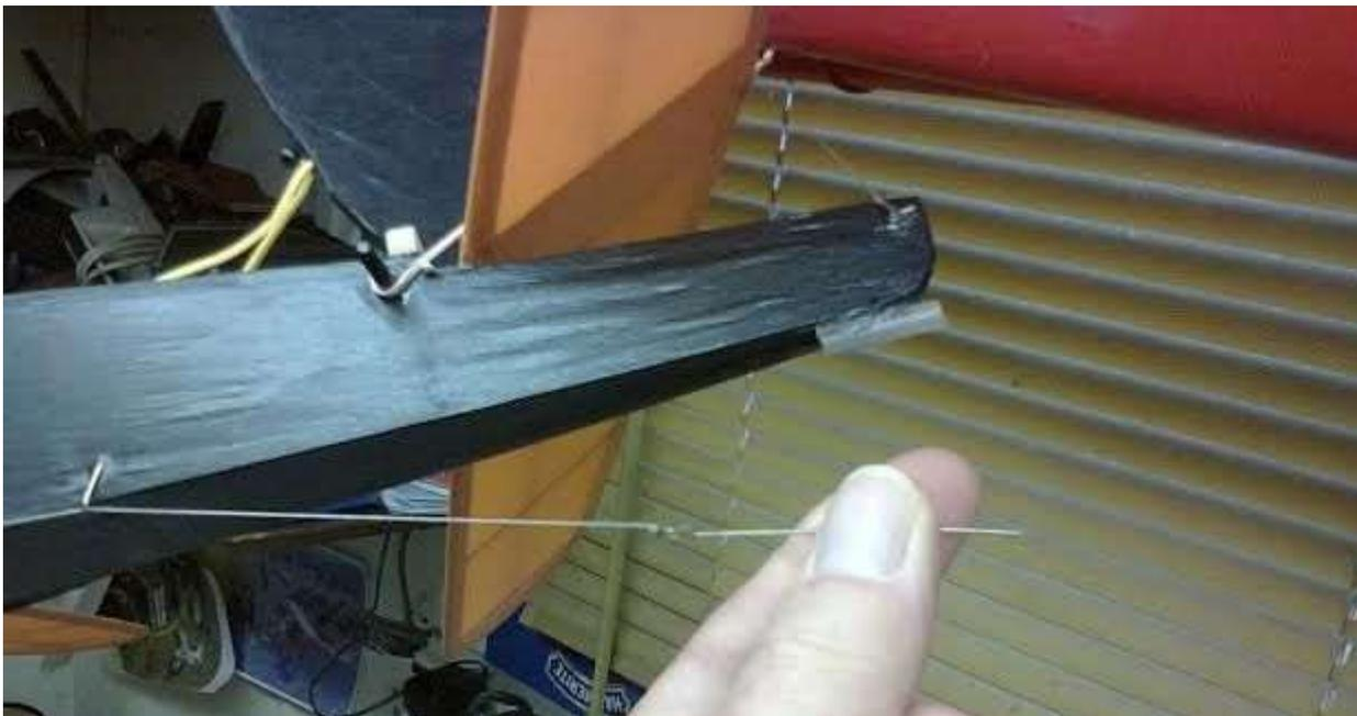
The picture above shows the grenade pin which sits in the tube with a short length protruding at the rear, over which the rubber band holding down the tailplane is looped.
