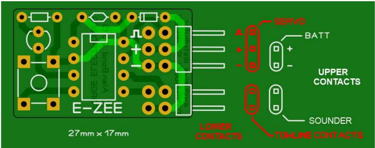
The battery lead usually coloured red/black, connects to the upper two pin header on the timer as shown in the image above and the D/T servo to the lower three pin header. Note the polarities of the battery and servo leads. The piezo sounder and towline contacts connect to the upper and lower two pin headers respectively and are not polarity sensitive.
