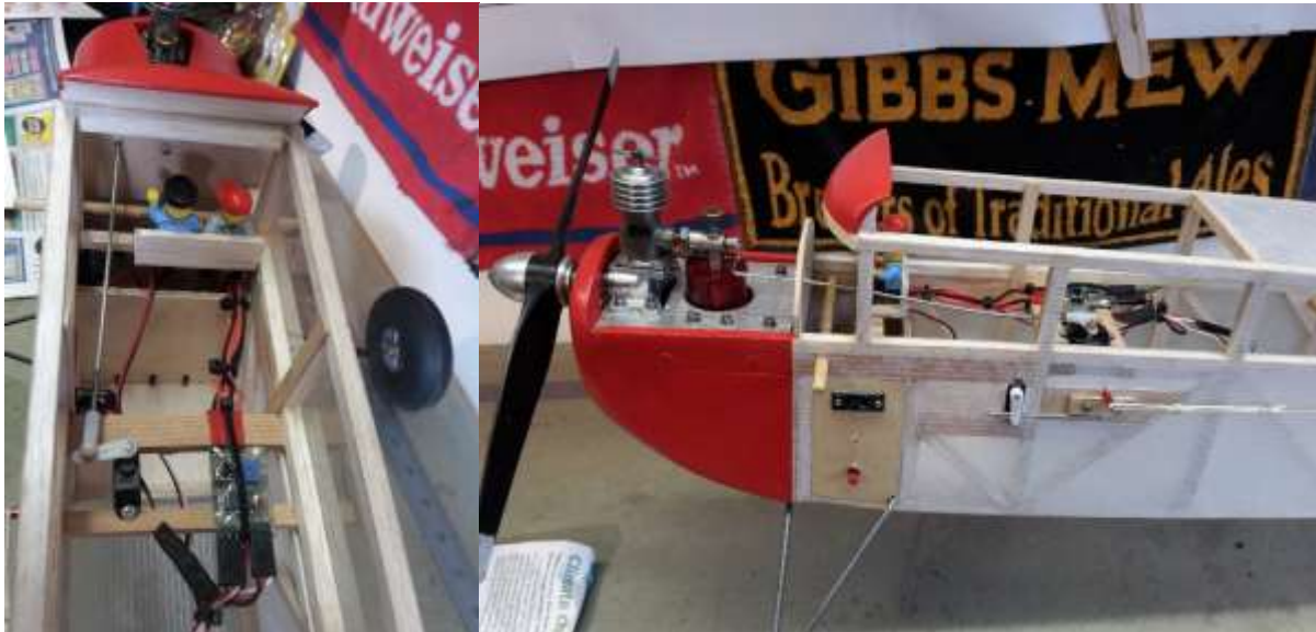
Timer board mounted inside the fuselage with LED and push switch extended to a plywood panel
