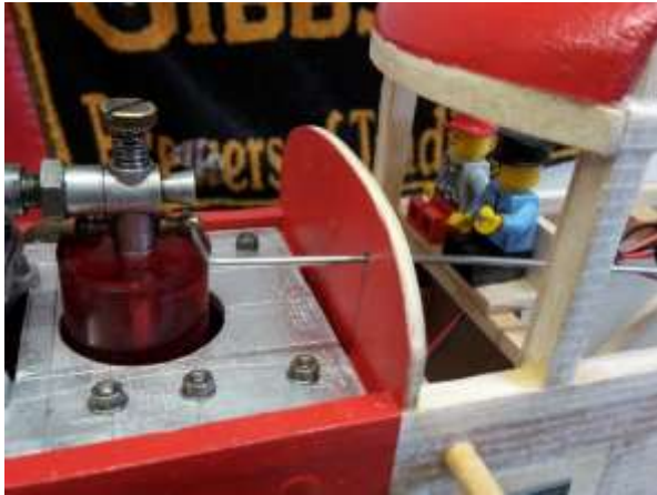
Simple pull rod connects to the original Comp Special Cut off – Note Lego men not necessary for correct operation
