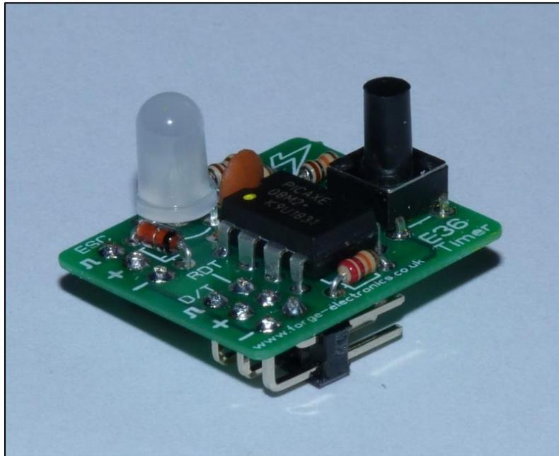
This is bespoke version of the E36 Competition Timer MK2 adapted to a customer requirement for F1E use. The former ESC output now drives a bunt servo instead. As the customer did not require the various configuration options of the E36 Timer these have been omitted to simplify the user interface – so only the bunt and DT servo timings can be adjusted.
