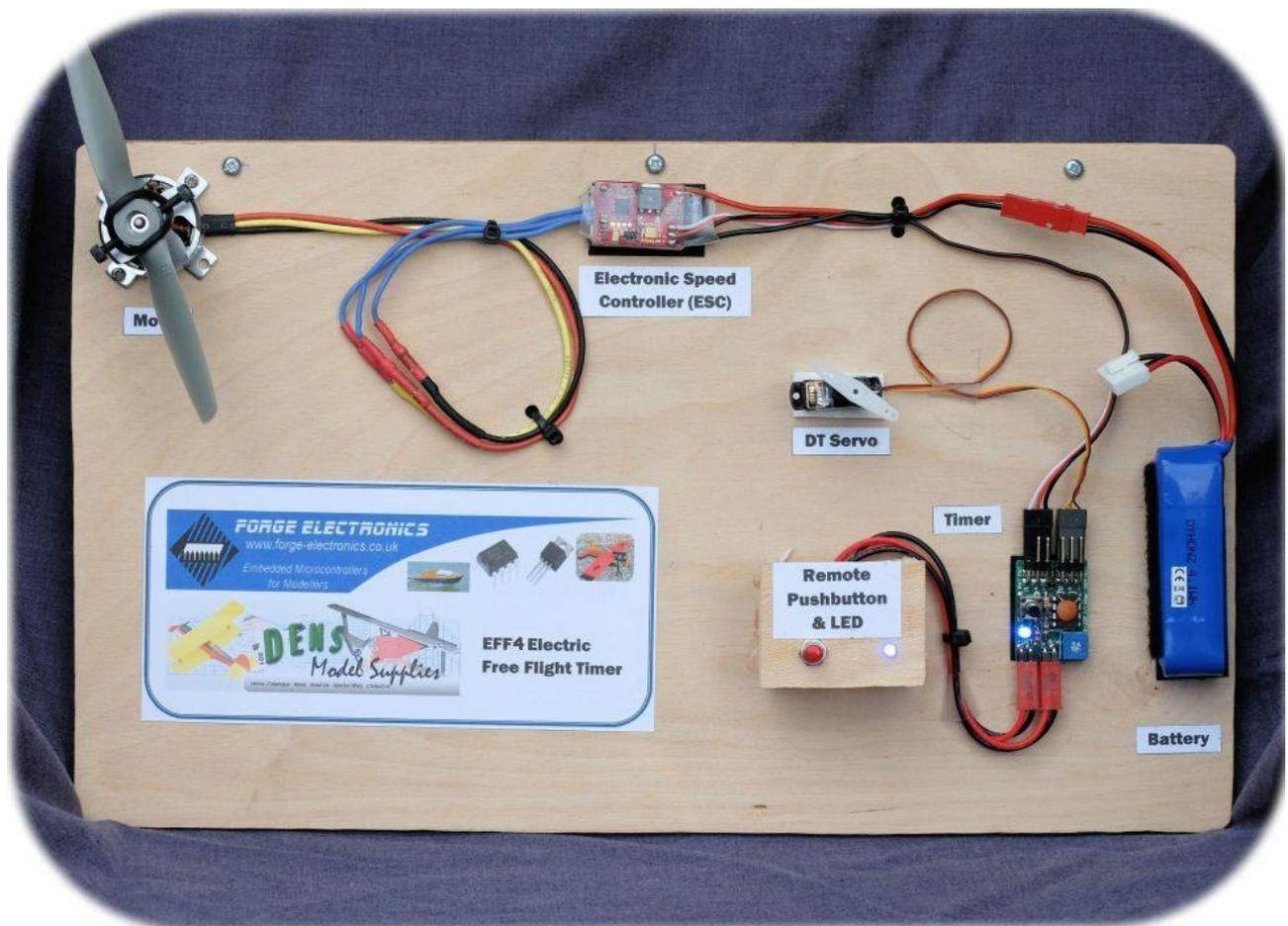
This image shows the system components, note that power does not flow through the timer. The timer is fed from BEC (Battery Eliminator Circuit) provided by the ESC and in turn sends signals to the ESC and the DT servo. **So the timer can be used with any size of motor/ESC/battery combination subject to the following warning**
