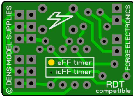
This PCB is also used for an IC Free Flight Timer version, which of course has different firmware, so to distinguish between the two variants, the PCB underside is marked with a yellow paint blob against the appropriate legend.
